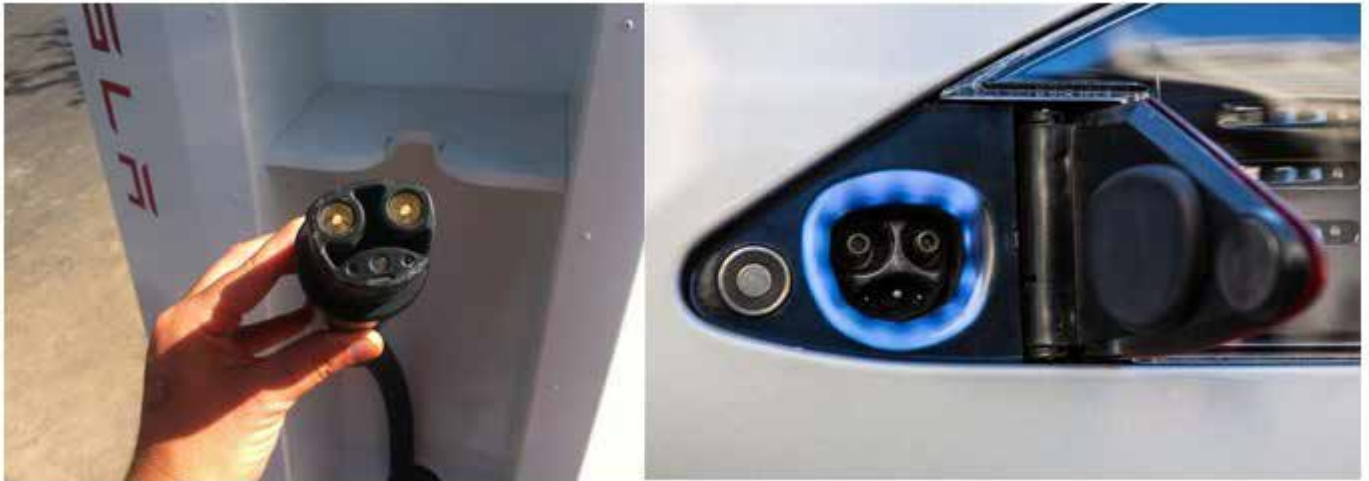
Tesla's proprietary Supercharger connects to the vehicle connector located in the tail light housing of the Tesla Model S. Courtesy of the Electric Vehicle Infrastructure Training Program.
